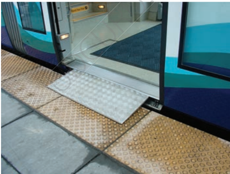
Wheelchair Ramp for a Tacoma Link streetcar (ภาพจาก https://commons.wikimedia.org/wiki/File:Wheelchair_Ramp_for_a_Tacoma_Link_streetcar.jpg )
