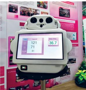
This is an innovative robot for the care of the older persons, the “Chula-Aree Version.” It can be controlled and commanded from a distance. It has the equipment to measure and record vital signs such as blood pressure, ECG, pulse, and temperature, for real-time diagnosis.
