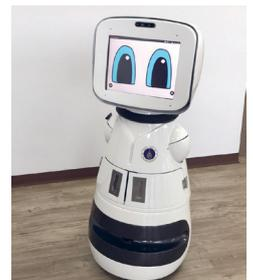
This is a robot used in diagnosis and treatment via telemedicine. It can perform routine tasks without the supervision of a clinician. Doctors or nurses can consult with people through the robot. The robot can measure the pulse, blood pressure, and heart rate, and help transport medicines and materials to persons with fever to reduce the risk of infection.
