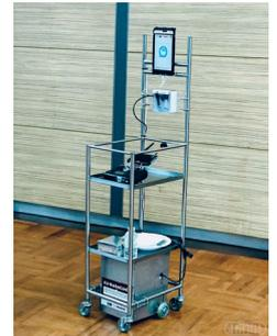
This is a robot used to deliver food and medical supplies from a distance.
